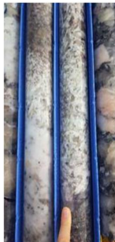
Some photographs of recent core with visible spodumene (left) and spodumene and lepidolite (right).
