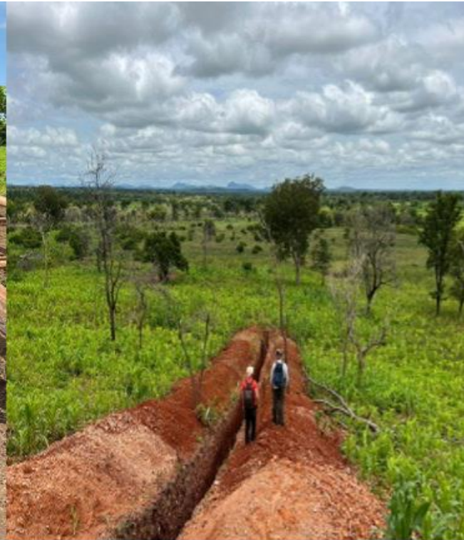
Trench across Spodumene Hill identified a pegmatite with an apparent width of >100m. Another three trenches were dug across the hill.
