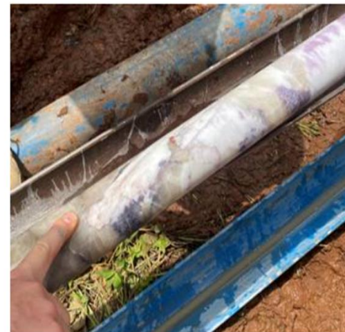
Some photographs of recent core with visible spodumene (left) and spodumene and lepidolite (right).
