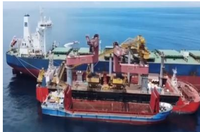
Gerald's TSVIO transhipper vessel loads Marampa Blue™ onto an Ocean-Going Vessel (OGV) for transportation to end users.
